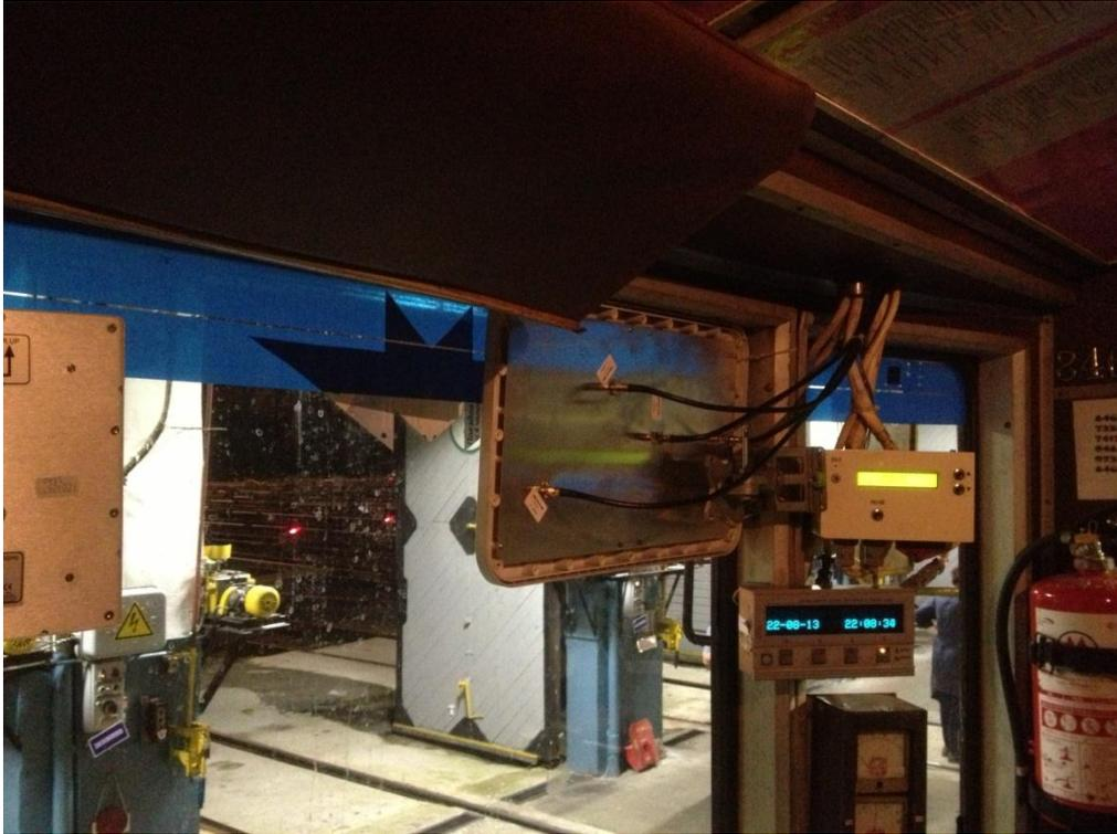
Pic. 2 WiBOX PA D4M5-20HVX MIMO 4x4 directional antenna and Cisco router installed inside the train.
