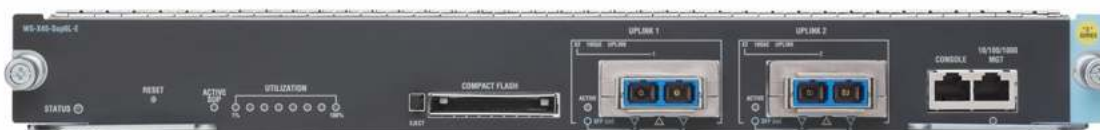
Figure 1. Basic Layer 3 Supervisor Engine 6L-E with TwinGig Support (Two 10 Gigabit Ethernet or Four Gigabit Ethernet)
