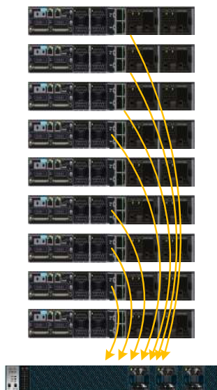
Figure 5. Star Topology, Using an XPS
